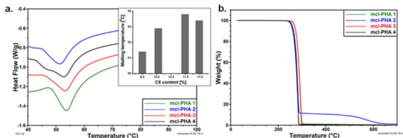
Fig. 7. (a) DSC thermograms of *mcl*-PHAs (inset: Melting temperature vs. C6 content in PHAs); (b) TGA curves of *mcl*-PHAs
