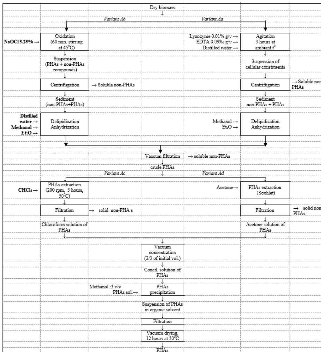
Fig. 1. Experimental variants for *mcI*-PHAs isolation from digested bacterial biomass
