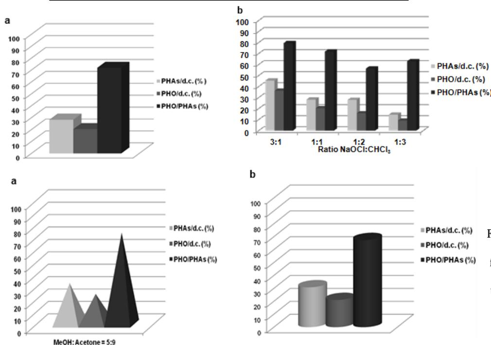
**Fig. 2.** (a) *mcl*-PHAs (PHO) isolation by enzymatic digestion of biomass followed by CHCl<sub>3</sub> extraction (AaAc variant); (b) Influence of NaOCl:CHCl<sub>3</sub> ratio of the extraction mixture on *mcl*-PHAs (PHO) isolation (AbAc variant with simultaneous digestion and extraction treatment)
