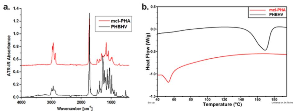
Fig. 6. (a) FTIR spectra of *mcl*-PHAs and PHBV; (b) DSC thermograms of *mcl*-PHAs and PHBV
